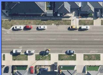
CENTRE LINE AND BICYCLE LANE LINE MARKING
